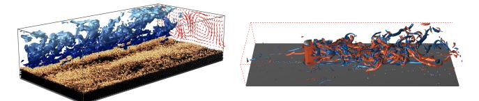
(Left) Open channel flow over a mobile sediment bed. (Right) Particle motion around a wallmounted cylinder over a smooth surface.
